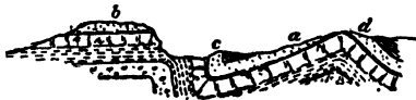
FIG. 74.—Section to show dependence of extent of outcrop on slope of the ground and dip of the beds. The same bed is wide at a and b , but narrow at c and d .
